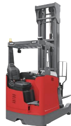
MFZ16/20 Seated Reach Truck Rated Capacity 1600/2000kg Max.lift height 12000mm
