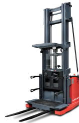
MHA13 Order Picker Rated Capacity 1360kg Max.ift height 9500mm
