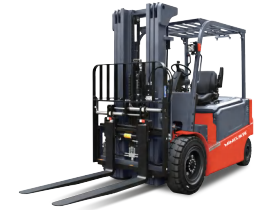
MK25/30 4-wheel Counterbalanced Forklift Truck Rated Capacity 2500/3000kg Max.lift height 6000mm
